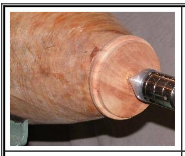
This shows the tenon, all cleaned up and nice and round and square. In a later photo you will see how far the piece actually moved out of round.
