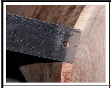
This is how deep the cut is on one side, and the chisel had not yet contacted the other side. It was a half inch out of round. Of course, the inside of the vase was that far out of round as well. I had left the walls a bit over 3/4" thick, so at the very most, just turning the piece back round again would leave it 3/8" or so thick.
