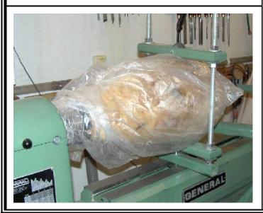
To leave a wet piece on the lathe overnight, I just put a bag around it. Have to in order to keep it from splitting. I suppose you could use Pentacryl or something like that too, but a bag is cheaper.
