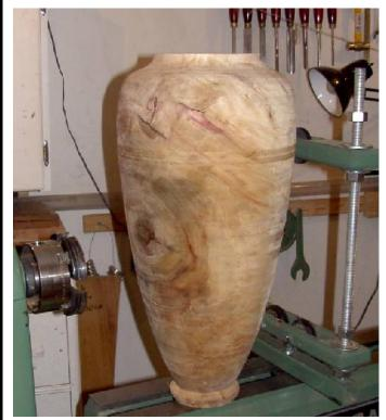
Rough turned and ready for waxing. The piece is about 1¼" thick and weighs 25 pounds. It is 23" deep on the inside. The rough blank was 26" and the piece is now 24½" and the largest diameter is still close to 16". I will coat it with sealer and set it aside – probably for a year or so before it is finished
