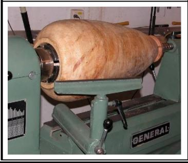
To re round the tenon, I make use of the #3 jaws in the Stronghold scroll chuck. I left a tiny ledge in the mouth of the rough vase in anticipation of this. The tailstock center is in the same center hole that was left when the piece was first turned between centers.
