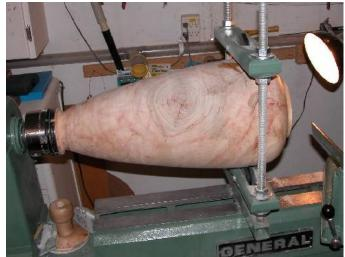
Now the piece is round and the steady rest is fitted into place so I can turn the inside.
