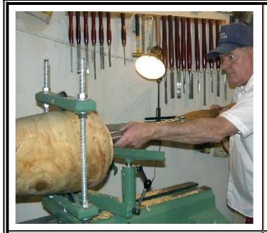
"Bigger Bugger" at work, also held in the armpit. I've found that the secret to cutting comfortably with these tools is to design the handle for this grip. The lathe has to be the proper height for it to work well. Although the photos look like I am watching the cutter, I am not. I go by feel and sound. Watching the cutter is a back killer. After three hours I have no back aches at all. Also not a single catch the whole time.
