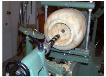
With a piece like this you have to drill a hole. I use a Jacobs chuck in the tailstock and an auger bit. This one is 1" by 8" and when I get to the maximum depth with this I use a 1¼" by 18" auger bit. With the extension of the tailstock quill to it's fullest extent I can drill down to about 23" with the auger. The auger bit would likely not work in dry hardwood, especially end grain.
