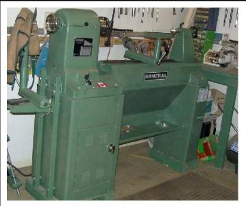
Whew! That's what the lathe is saying. All cleaned up, the nicks and scratches repainted, the ways cleaned and oiled. Ready for the next one.
