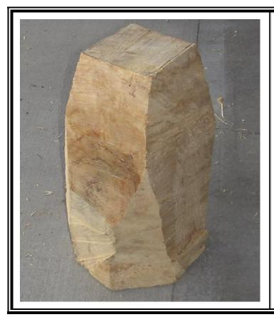
This is the box elder blank. Originally it was 16" square by 26" in height. I took the corners off and tapered it to reduce the weight as much as possible. After all, it had to go down into the basement. The blank, this way, weighed about 175 pounds.
