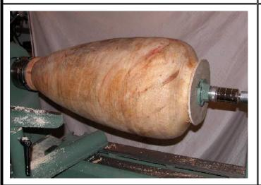
Now the scroll chuck holds the trued up tenon firmly, while the jam center steadies the vase and centers the mouth. The piece has warped far out of round - it is actually oval, and it has to be round again before I can use the steady rest. This is how I set it up
