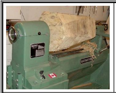
Blank mounted on the lathe between centers. Note the compass circle scribed on the end? The center point of the circle is where I drive home the spur center with a brass hammer to avoid damaging the center.
