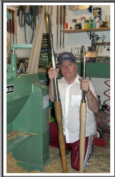
The tools of the trade. In my left hand is the "Big Bug" as Del Morrisette named it. It can handle down to 18" maximum, although I seldom go more than 14" or so with it. In my right hand is the "Bigger Bugger" a behemoth of  $1\frac{1}{2}$ " diameter, telescopes from 48" to 60" overall and heavy - 35 pounds. Has to be to go to 24" depths. Both of these use the #3 Oneway Termite tip, a ring cutter.
