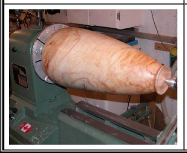
The vase sat for close to a month to complete its movement, and then was remounted and the outside trued up again.
