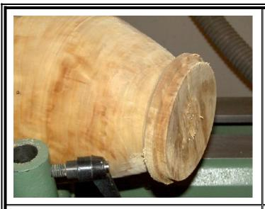
The tenon, about 4½" in diameter is for the #2 jaws for the Stronghold chuck.
