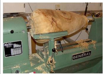
Turned to rough outside shape with a tenon on the tailstock end.
