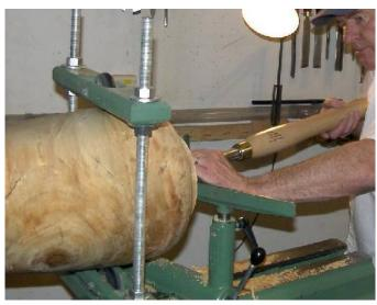
"Big Bug" at work, held under my arm. This piece is being turned cross grain, and the Termite is best at end grain. I rarely get a plugged cutter on end grain, but this was a bit more difficult. The fine shavings from every revolution across the end grain tends to build up in the cutter when cutting this very wet wood.
