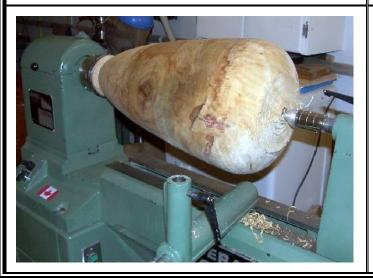
The tailstock center cone goes right into the hole left by the spur center. The reason for using the Stronghold and the tailstock is to turn the outside shape more precisely and to ensure it is perfectly round and centered where the wheels of the steady rest will run.
