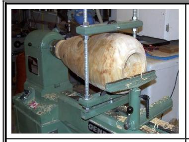
In the steady rest. The rest was set up with the tailstock in place to ensure the piece will run dead true.
